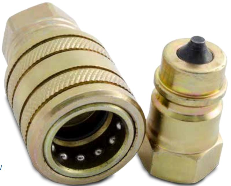
*Joint of 1/2 configured to flow rate up to 65L, with starter's tempered pin, internal seal with VITON 90 Shore (NOVA HIDRÁULICA EXCLUSIVE), temperature up to 150C, recommended working pressure of 180 Bar, test pressure of 250 Bar, starry diffuser reaching higher flow rate.*
