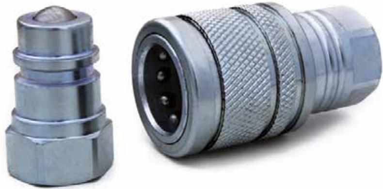
*Configured joint to flow rate up to 55 l/min, activation by sphere chrome steel, no internal seals, which enables work without damage to the sealing system. Recommended working pressure at 200 Bar.*
